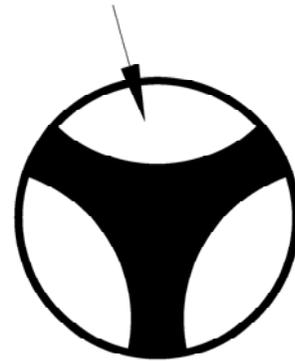
CROSS SECTION OF PUMP BUSHING
