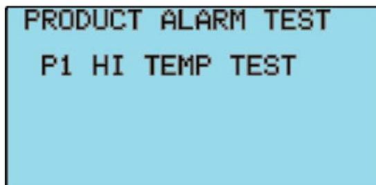
This screen will be displayed when a test is active. To end a test press the ENT key to move the cursor to the TEST data field and use the Up or Down Arrow key to scroll through the tests until "NO TEST SELECTED" is displayed. Press the ENT key to end the test.
