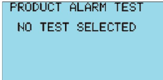
Press the ENT key to move the cursor to the NO TEST SELECTED data field. Use the Up or Down Arrow key to scroll through the tests. When the correct test is displayed press the ENT key to start the test. Press the ESC key to return to the System Status screen.
