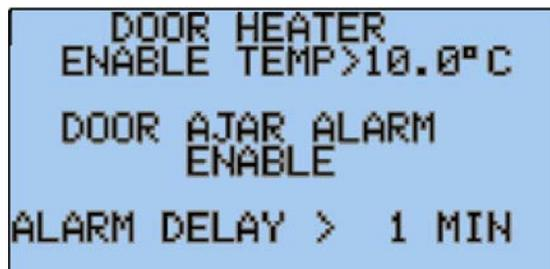
Factory Default Setting: Door Heater Enable Temp > 10.0°C
