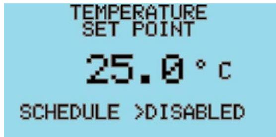
**Note:** If the schedule is enabled the temperature will be set through the ramp and soak schedule. To disable the ramp and soak schedule press the ENT key to move the cursor to the schedule field. Use the Up or Down Arrow key to disable the schedule. Press the ENT key and the cursor will move to the upper left hand corner and the set point will be visible. A full explanation of the ramp and soak schedule follows.
