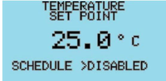
Press the Enter key to move the cursor to the schedule field. Use the Up or Down arrow key to enable the schedule. Press the Enter key and the first of 21 Ramp and Soak screens will be displayed.
