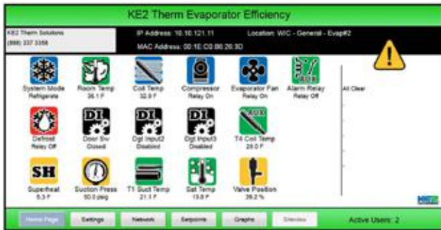
Screen shot of a single Evap connected through Smart Access.
